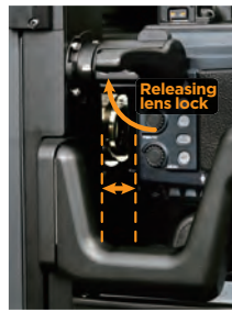
Sliding back while camera is mounting on the sled
